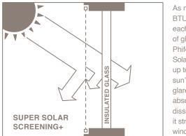
As much as 230 BTUs can fall on each square foot of glass. With Phifer Super Solar Screening+, up to 90% of the sun's heat and glare is reflected, absorbed and dissipated before it strikes the window surface.
