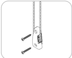
If mounting to wood or metal, drill holes through your marks with a 1/8" drill bit. Then secure the Tension Device using the provided Phillips panhead screws.
