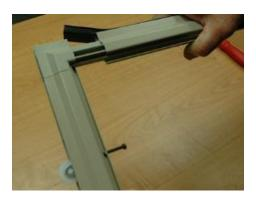
B) Assemble side rails to top rail, tap corners into place if needed
