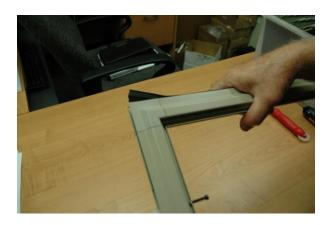
C) Assemble side rails to bottom rail, tap corners into place if needed
